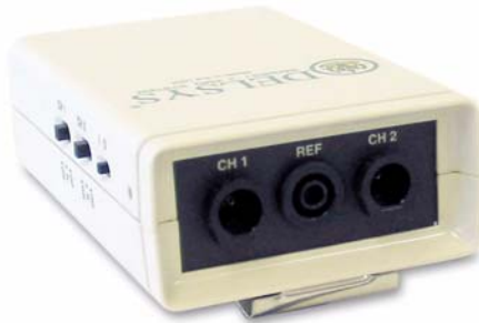
Figure 3. Bagnoli-2 Main Amplifier Unit
