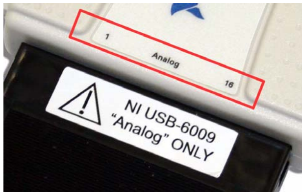
Figure 12. Ensure the Cable is connected to the “Analog” input side of the USB-6009 device.
