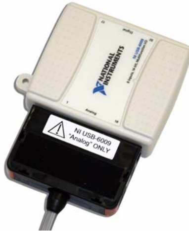
Figure 11. Connecting the Output Cable to the USB-6009.
