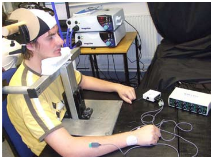
The experimental setup: TMS causes a muscle contraction that can be recorded using surface electromyography.
