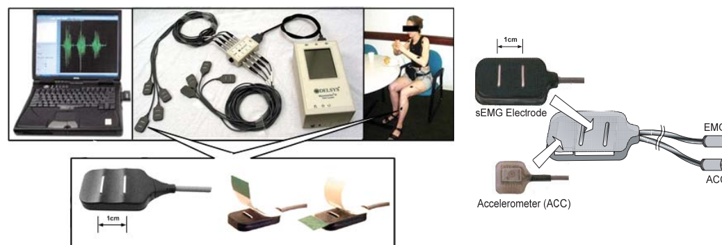
Figure 2. (Left) Hardware developed by research team members to acquire and store up to 16-channels of EMG or ACC signals. Sensors are connected to a body-worn repeater (middle photo) which wirelessly transmits the data to a PC base station. Details of the surface EMG electrode innovation are seen in the callout. (Right) Prototype hybrid sensor combines EMG and ACC signal detection.
