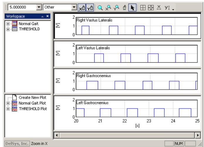
*Figure 2B: Activation intervals for each of the muscles from the normal gait obtained using the Threshold calculation.*
