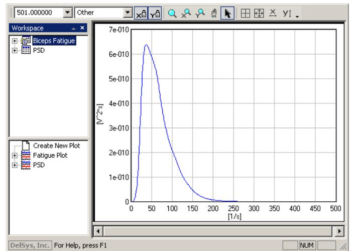
*Figure 4B: PSD for the EMG data from the biceps. The contribution of power from each frequency can be visualized.*
