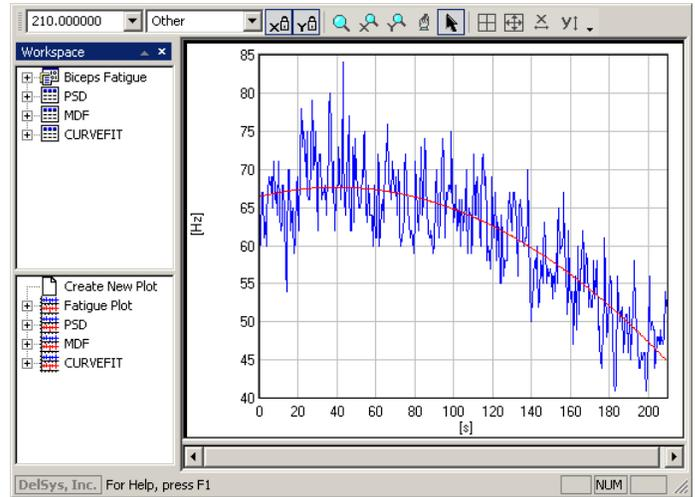
*Figure 5B: Median frequency of the biceps EMG data as a function of time along with a curvefit to quantify the decrease in median frequency.*
