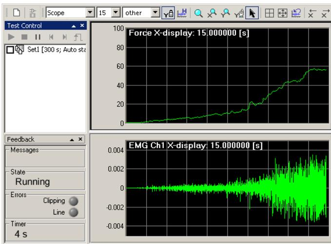
*Figure 1A: Force output from the first dorsal interosseous muscle of the hand recorded with the corresponding EMG activity. It is clear visually that the amplitudes are roughly proportional.*
