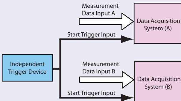
Figure 4: All data acquisition systems are started by an independent device that issues a common Start Trigger Input.
