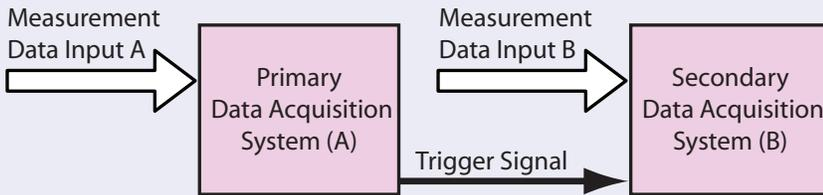
Figure 3: The Primary System issues a Start Trigger Output signal which controls the Secondary System. It may be necessary to condition the signal so that it is interpreted correctly.
